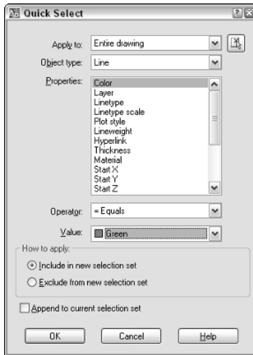
Figure 5-1: Quick Select allows you to filter objects by a single property.
